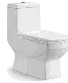
CB.12.0007 Washdown One-piece Closet Size: 740x380x750mm S-trap, 250/300mm P-trap, 180mm Roughing-in
