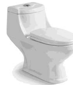
CB.12.0032 Washdown One-piece Closet Vitreous China Size: 700x370x650mm S-trap, 250/300/400mm Roughing-in P-trap, 180mm Roughing-in
