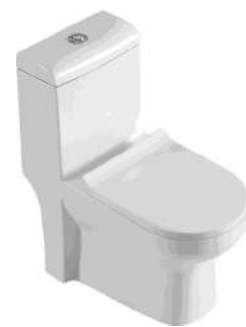
CB.12.0008 Rimless One-piece Toilet Size:780x365x705mm S-trap,200mm,250mm Roughing-in P-trap,180mm Roughing-in
