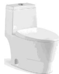
CB.12.0131 Washdown One-piece Toilet Size: 680x400x760mm S-trap, 250mm/300 mm Roughing In P-trap, 180mm
